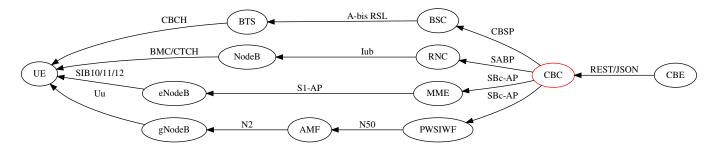
Figure 1: Role of the CBC inside the 3GPP network architecture (3GPP TS 23.041 §3)
