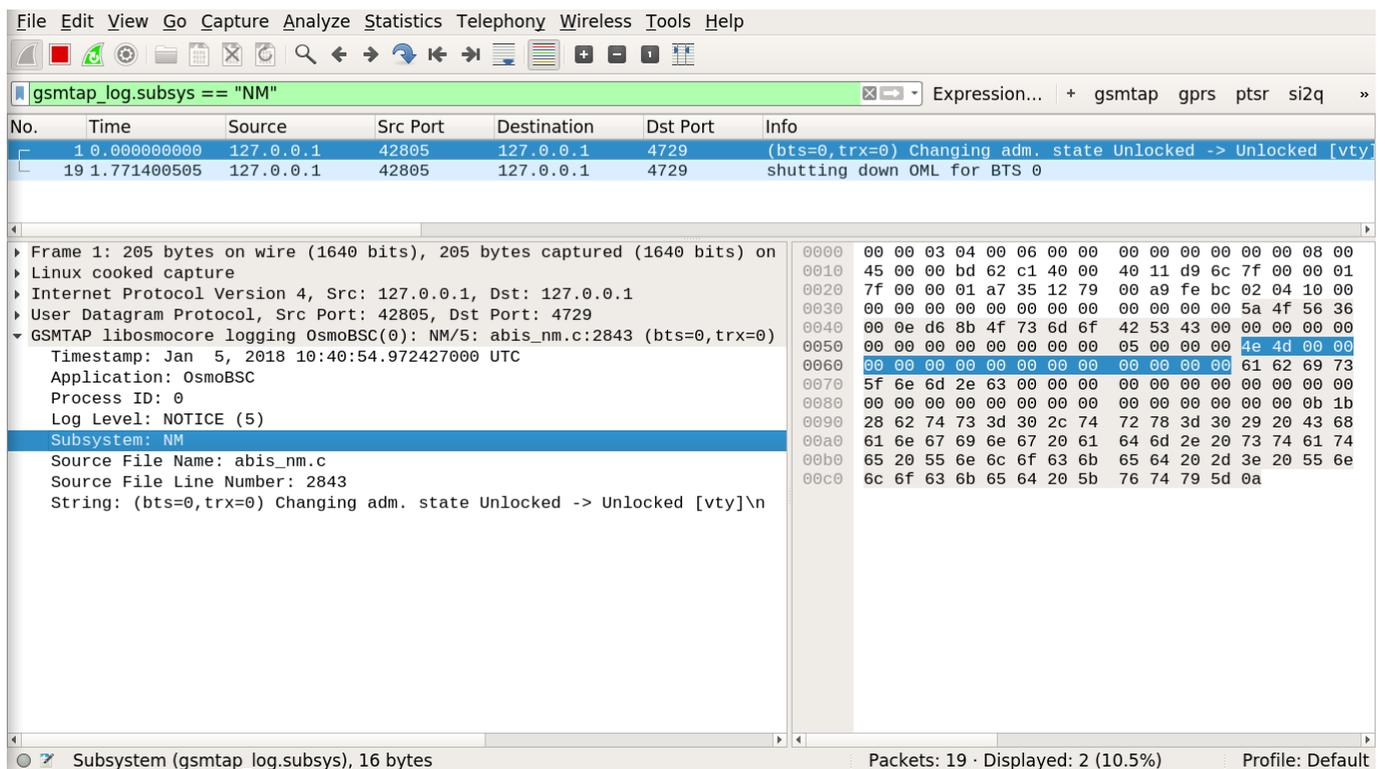
Figure 2: Wireshark with logs delivered over GSMTAP
