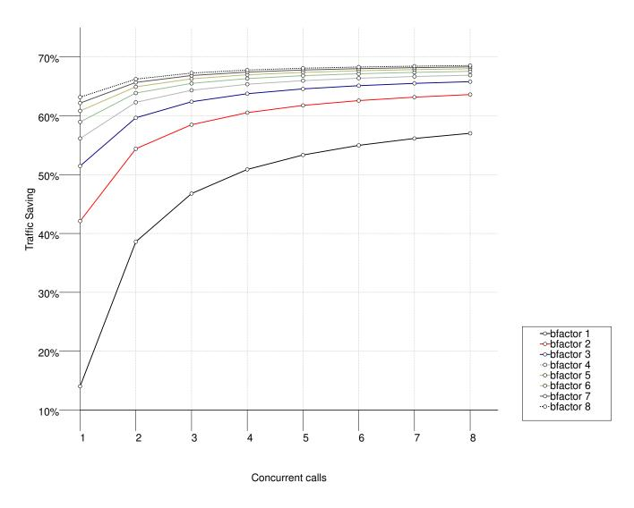
The results show a saving of 15.79% with only one concurrent call and with batching disabled (bfactor 1), that quickly improves with more concurrent calls (due to trunking).
