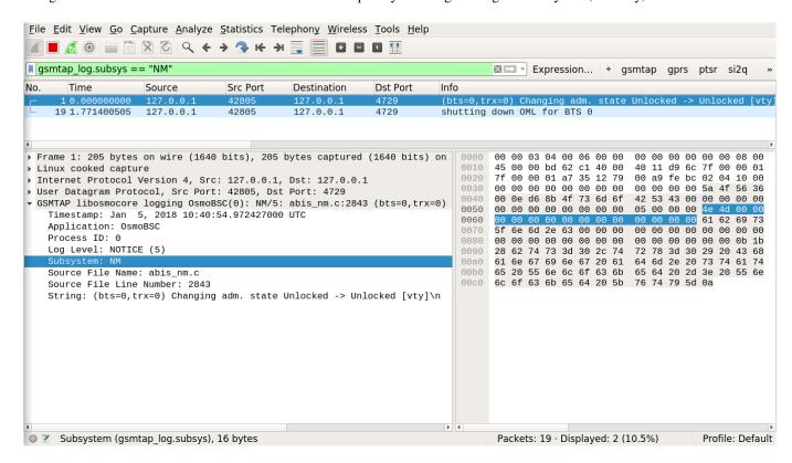
Figure 2: Wireshark with logs delivered over GSMTAP
