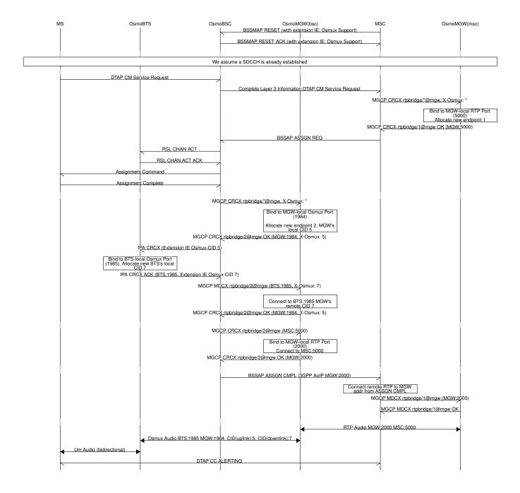
Figure 12: MO-call with Osmux enabled on Abis
