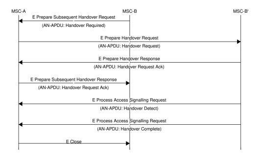
Figure 31: E Subsequent Handover (Normal Case)
