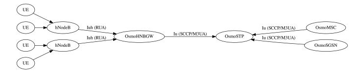
Figure 4: Simple signaling network for 3G (UMTS)
