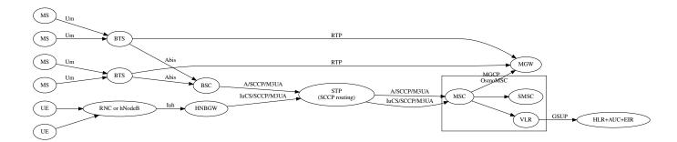
Figure 1: Typical GSM network architecture used with OsmoMSC
