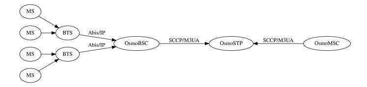
Figure 3: Simple signaling network for 2G (GSM)
