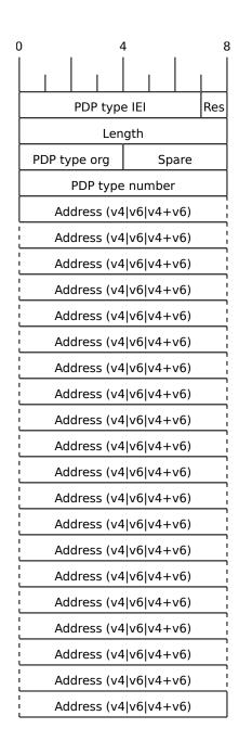
The spare bits are left undefined. While 3GPP TS 29.060 7.7.27 defines them as 1 1 1 1, there are MAP traces where these bits are set to 0 0 0 0. So the receiver shall ignore these bits.
