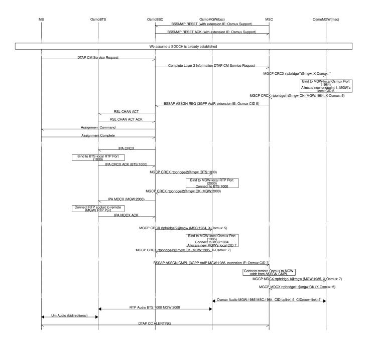
Figure 6: MO-call with Osmux enable on 3GPP AoIP
